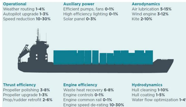
Figure 1: Potential fuel use and CO<sub>2</sub> reductions from various efficiency approaches for ships (International Council on Clean Transportation (ICCT), July 2013). Long-term potential for increased shipping efficiency through the adoption of industry-leading practices.
