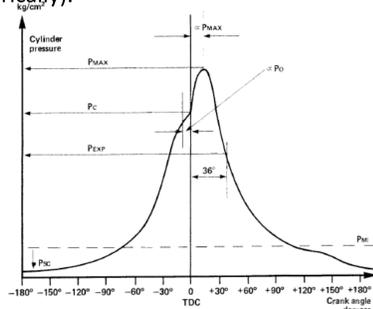
Lower than expected cylinder pressure generally means that engine settings are not optimal or its components may be faulty. In practice, other engine process parameters such as pressures, temperatures, turbocharger speed, etc. are monitored to support the above analysis.
