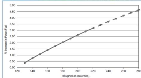
Hull fouling and roughness have significant impact on ship resistance
