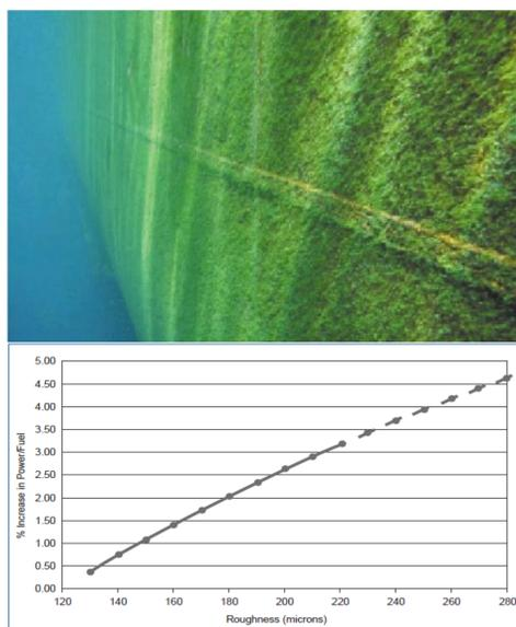
Hull fouling and roughness have significant impact on ship resistance
